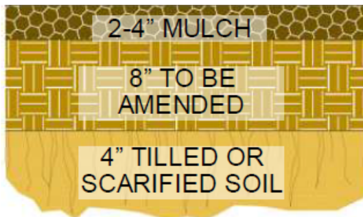
Figure 3 Lawn or landscape garden, the same generalized cross section of loosened and amended soils apply.
